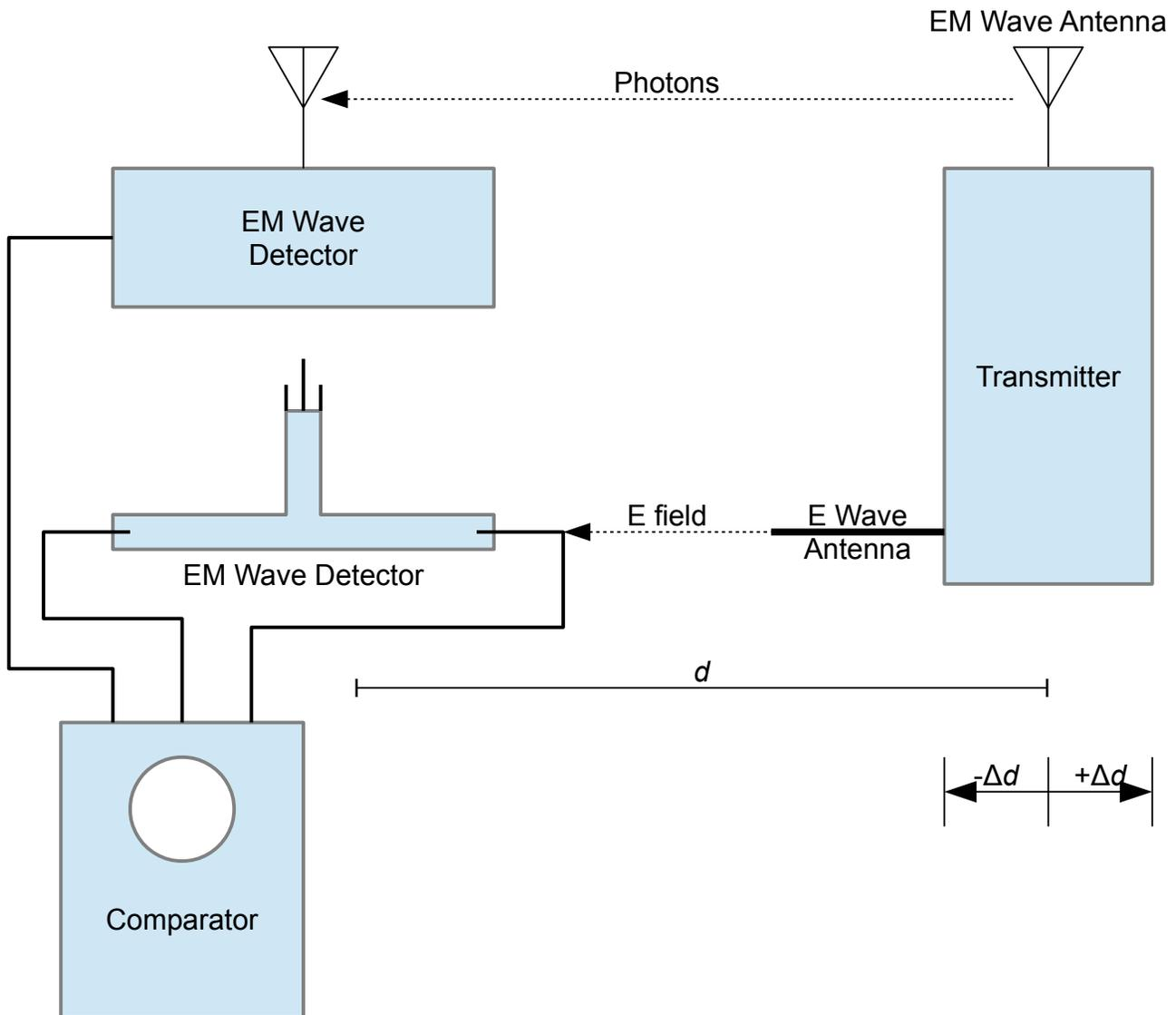
Figure 1: Experimental Apparatus for the Determination of  $t = (t_{em} - t_E) \begin{cases} = 0 \\ \neq 0 \end{cases}$
