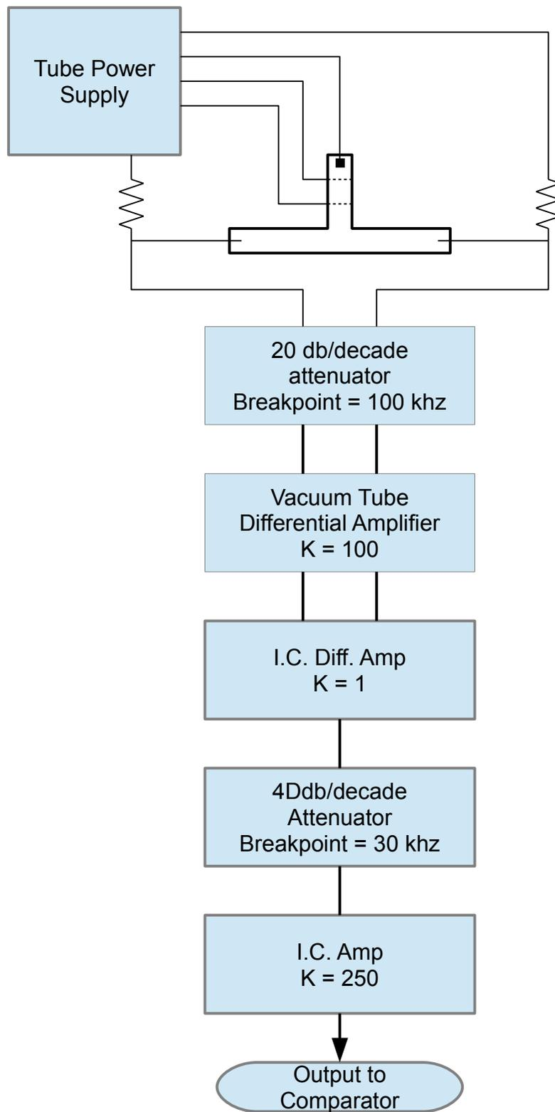
Figure 3: E Field Detector Tube and Associated Systems
